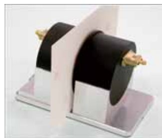
A sample setting of a resonant cavity for a flat panel
