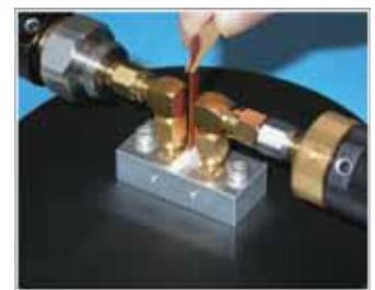
A sample setting of 2-10GHz resonant cavity
