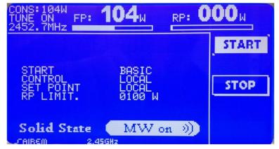
All operating parameters and control status, as well as any possible fault, forward power and reflected power are displayed on the screen. The forward power set-point is pre-displayed before starting.
