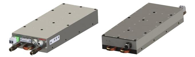
The MMS200WSMXPR2IR is a high power solid state module generator for the ISM band at 2.45GHz. It provides a CW output power adjustable from 0 to 200 W at frequencies ranging from 2400 MHz to 2500 MHz. This generator is designed for scientific and industrial applications, to be used with one or multiple MW applicators, to assure high reliability and small footprint. The protection against high reflected power and the measurement of reflected power are performed via a built-in isolator.
