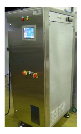
The GKP 24KP 18GHz consists of a single cabinet housing the power supply and the RF circuits. The cabinet can be easily transported on a pallet or fork-lift truck.
